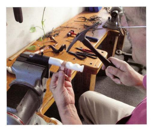
Turn it 180 degrees and hammer the other side the same way. Work at a steady speed; if you rush, an undesired fold can develop. Hammer rows with each blow slightly overlapping that of the previous row until the piece of metal is completely hammered. Once you have finished hammering the entire piece, anneal.
